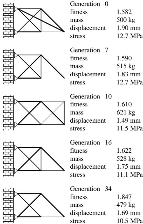
Fig. 24: Cantilever 15-Bar Truss
