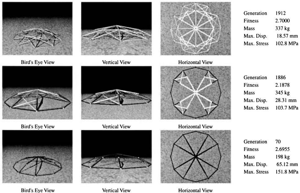
Fig. 44: Obtained Solutions of Sphere Hybrid Dome
