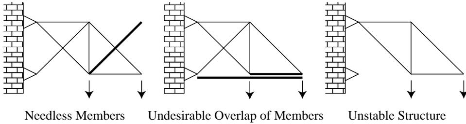
Fig. 1: Undesirable Structures
