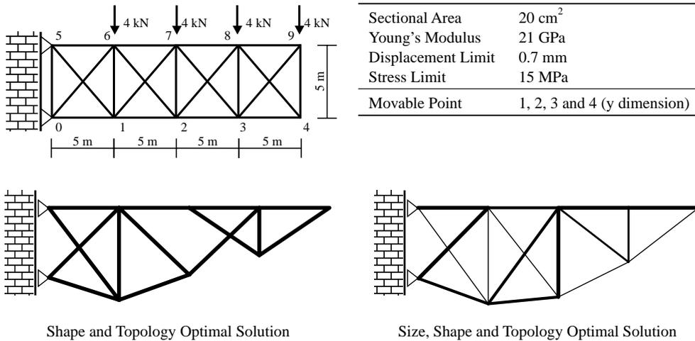
Fig. 25: 21-Bar Cantilever Truss
