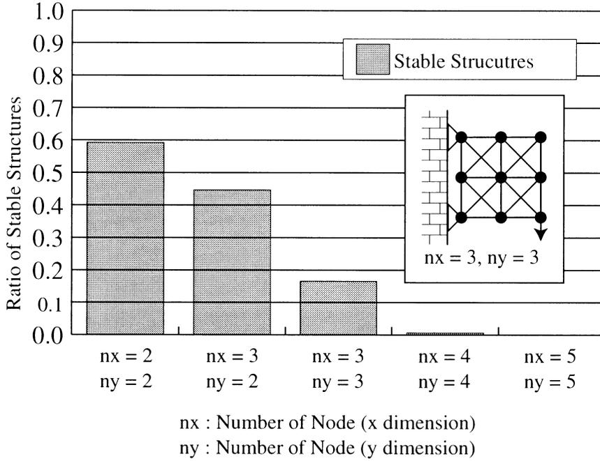
Fig. 2: Probability of Producing Stable Structures
