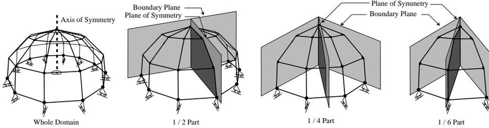
Fig. 39: Sphere Frame Dome
