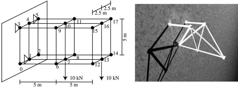
Fig. 26: 3-Dimensional Cantilever Truss
