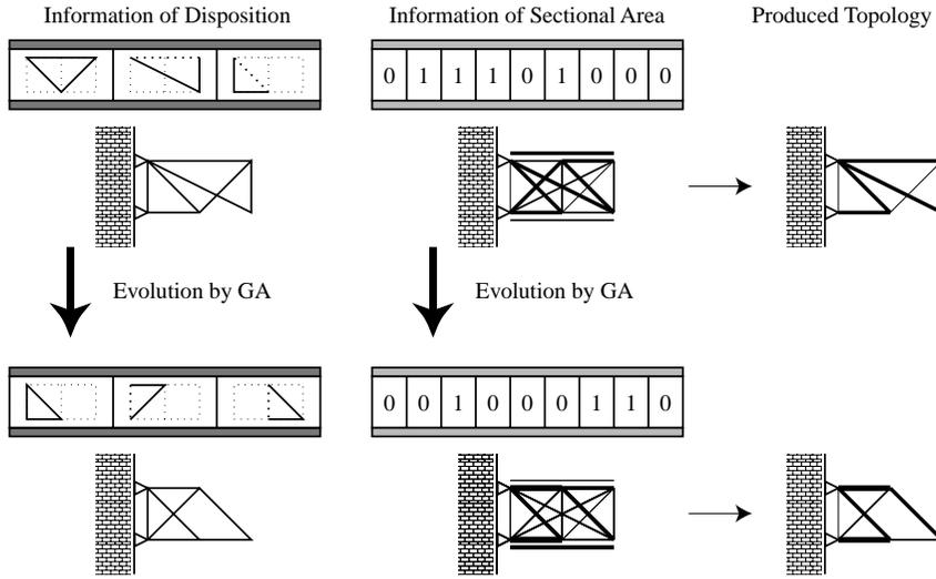
Fig. 19: Expression of Truss Topology by Plural Variables
