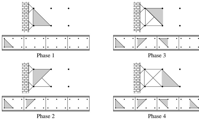
Fig. 3: Truss Topology Consisting of Triangles
