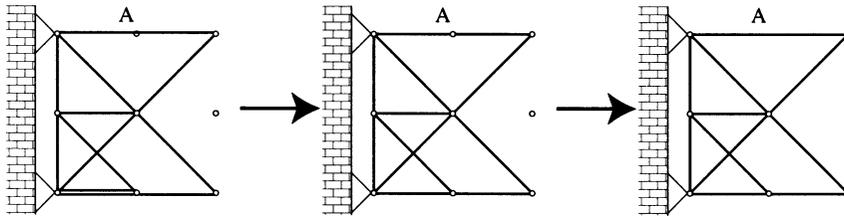
Fig. 9: Transforming to the Structure from the Combination of Stable Elements
