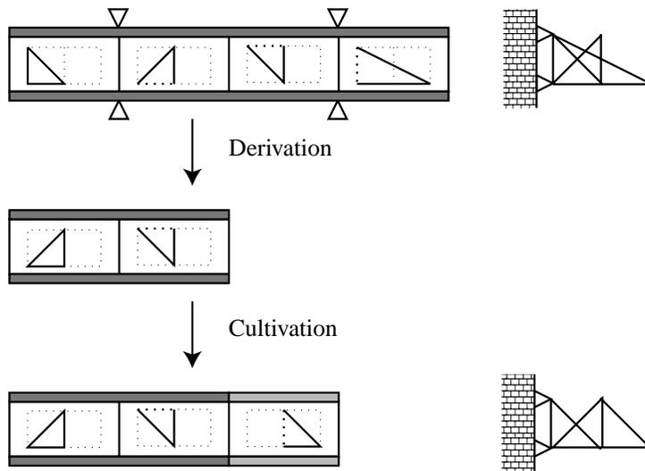
Fig. 18: Mutation Based on Triangular Element
