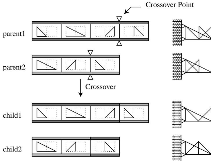
Fig. 17: Crossover Based on Triangular Element
