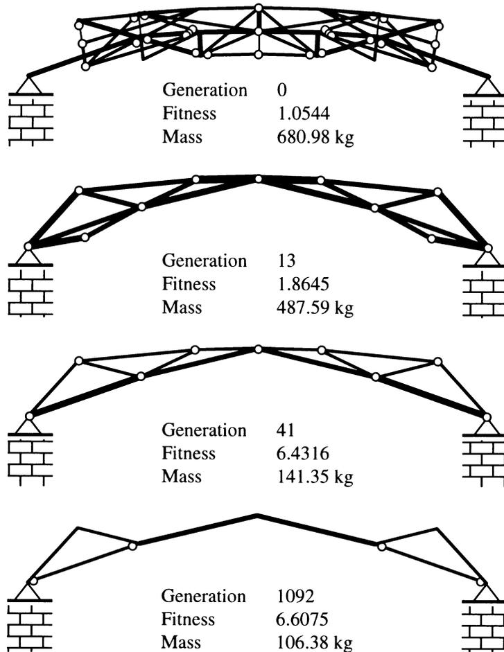
Fig. 42: Obtained Solutions of Planer Hybrid Arch
