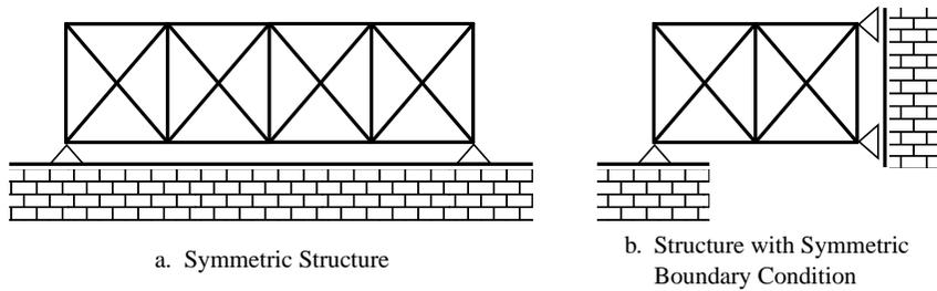
Fig. 14: Structural Analysis with Symmetric Boundary Conditioner
