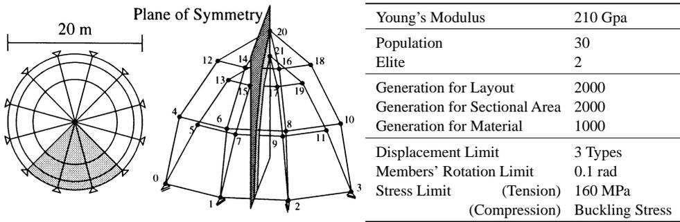
Fig. 43: Sphere Hybrid Dome
