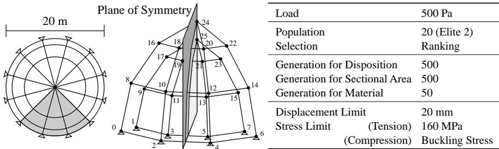
Fig. 27: Sphere Truss Dome
