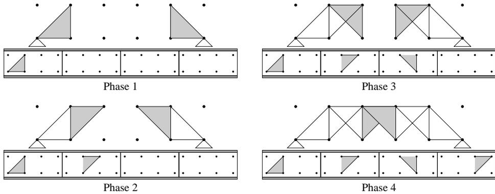
Fig. 16: Generation of Truss Topology with Topological Symmetry
