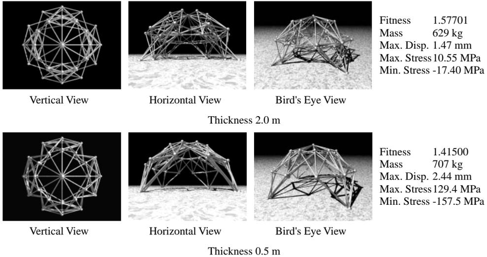
Fig. 31: Solutions with Difference of Thickness
