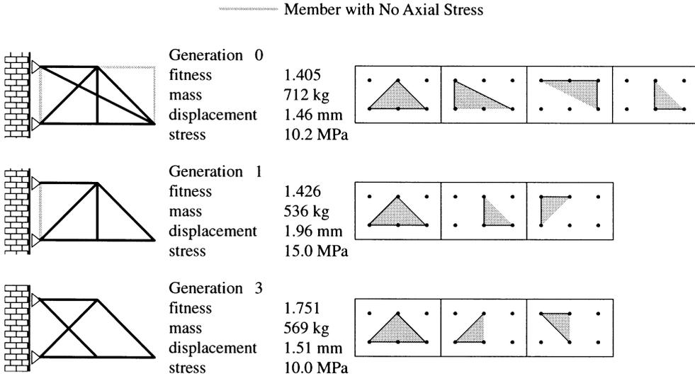
Fig. 23: Cantilever 15-Bar Truss
